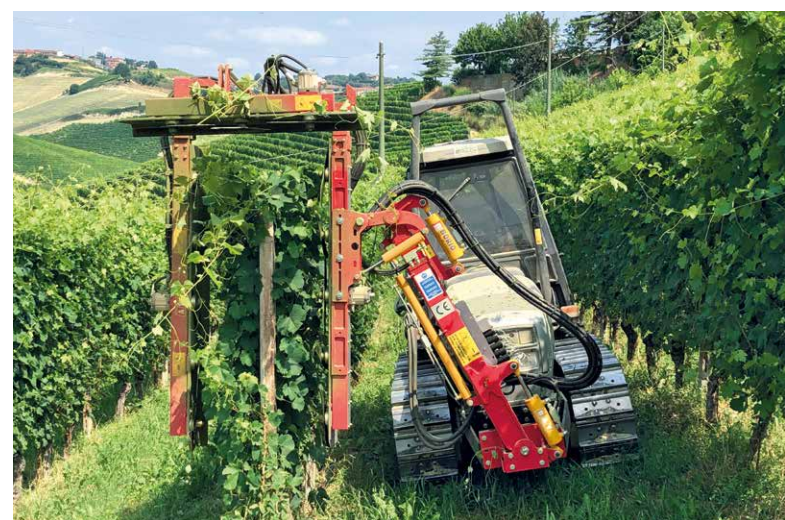
VERSION WITH PISTON FOR EXTERNAL VERTICAL BAR RETRACTION (0-90°) + ANTI-SHOCK SAFETY SPRING.
